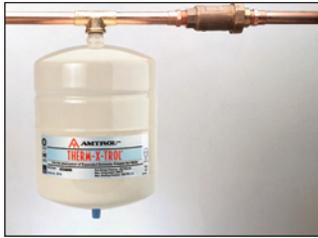
As the water is heated, thermal expansion occurs. Pressure increases until the relief valve opens and the expanded water spills from the water heater. This spillage results in wasted energy and a potential safety hazard. (See Diagram 1)
