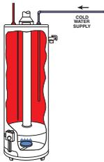
In a 40-gallon water heater, water being heated will end up expanding to about 40.53 gallons when the desired temperature is reached.
