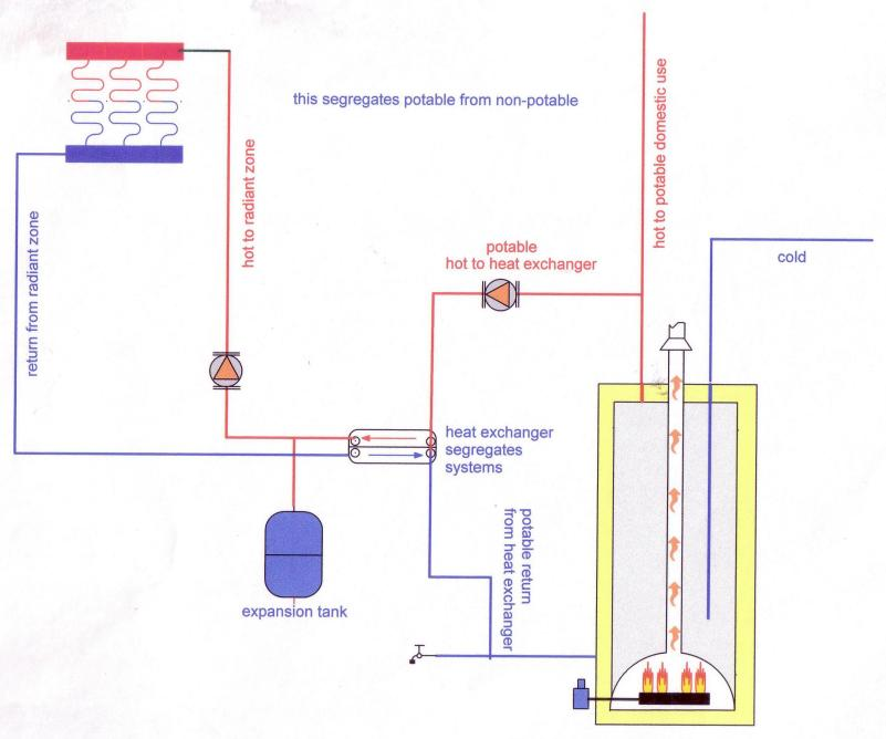
closed system off a water heater
